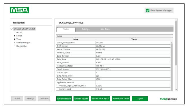
NOTE: The FieldServer Manager tab (see image above) allows users to connect to the Grid, MSA Safety's device cloud solution for IIoT. The FieldServer Manager enables secure remote connection to field devices through a FieldServer and its local applications for configuration, management, maintenance. For more information about the FieldServer Manager, refer to the MSA Grid - FieldServer Manager Start-up Guide.
