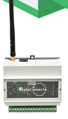
PG703 gateway can seamlessly connect one or many OEM devices into BMS networks including like BACnet IP, BACnet MSTP, Modbus TCP/IP, Modbus RTU, SNMP, MQTT, JSON, OPC DA, Minerva, OPC UA, FTP Client, SQL, Agilent, Hochiki EN, Email, SMS, Telnet, Veeder root, Hochiki MC and many more. It is a Bi-directional Converter that can be configured as a client and/or a Server on either protocol interface.
