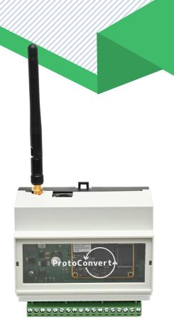
PG701 single wireless gateway can seamlessly connect one or many OEM devices into BMS networks including like BACnet IP, BACnet MSTP, Modbus TCP/IP, Modbus RTU, SNMP, MQTT, JSON, OPC DA, Minerva, OPC UA, FTP Client, SQL, Agilent, Hochiki EN, Email, SMS, Telnet, Veeder root, Hochiki MC and many more. It is a Bi-directional Converter that can be configured as a client and/or a Server on either protocol interface.
