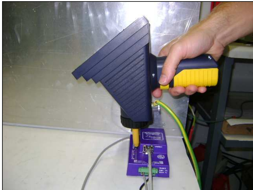
IEC 61000-4-2: Electro Static Discharge test set-up
