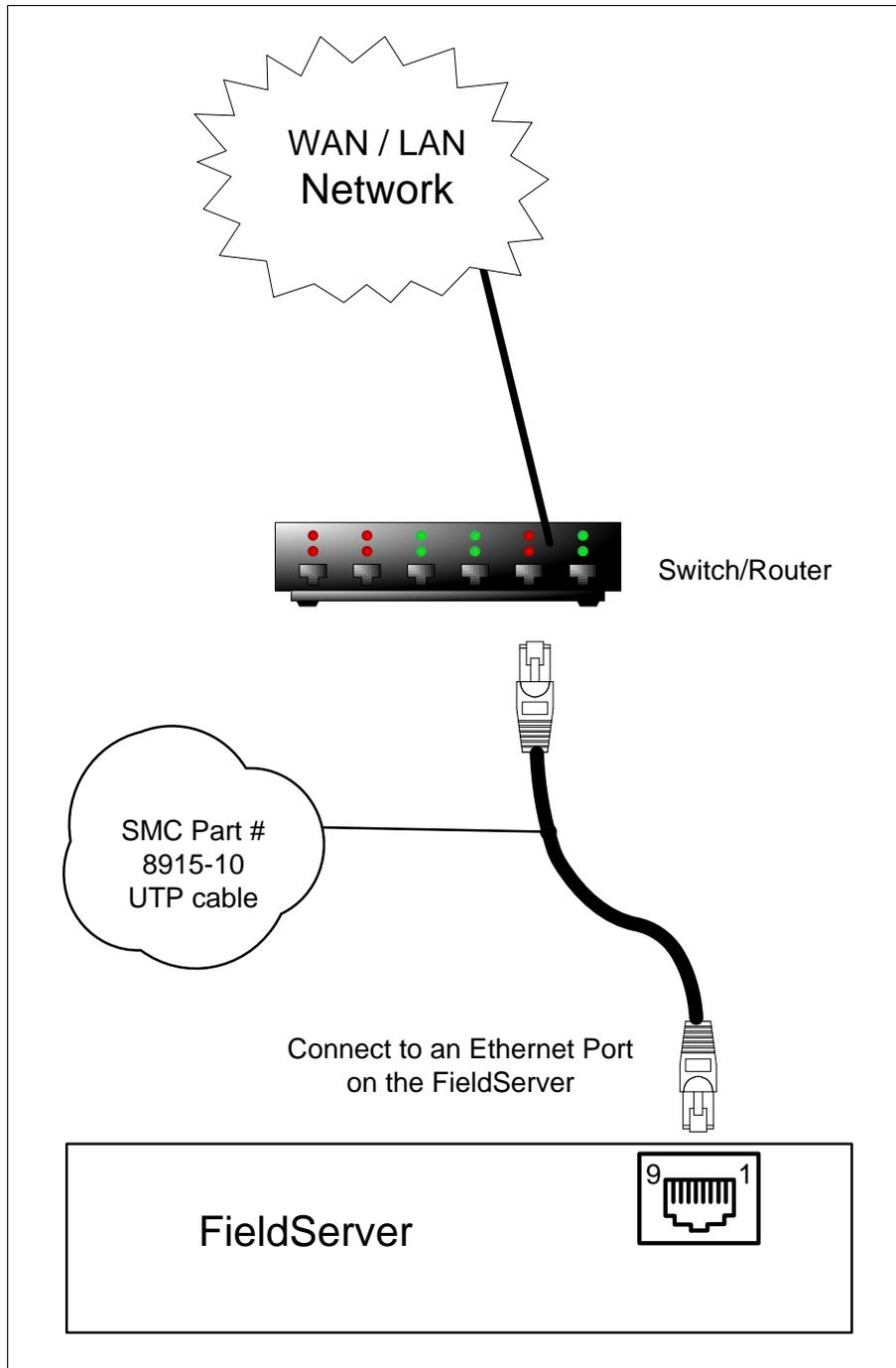
The Ethernet connection can be achieved using a switch or crossover cable. The driver will support all Ethernet connections on a local area network (LAN) or wide area network (WAN) including internet connections and crossover cable connections.
