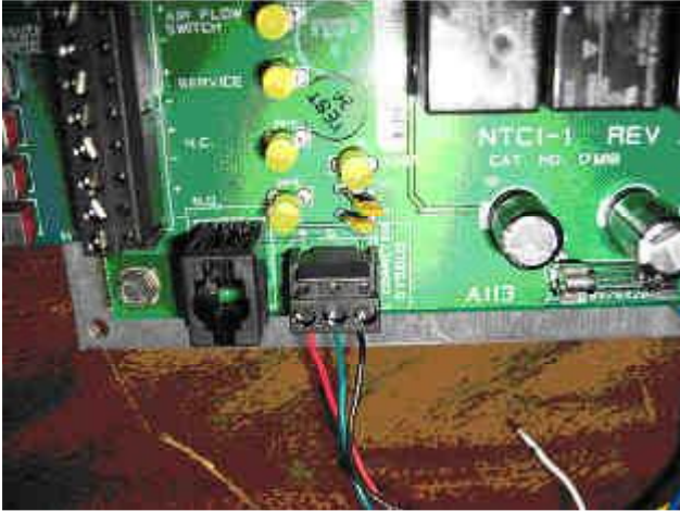
Photo of a terminating connection (no additional devices connected) on a Lennox NTC1-1 Board. A number of Lennox control boards have S-Bus connections which are labeled in a similar way.
