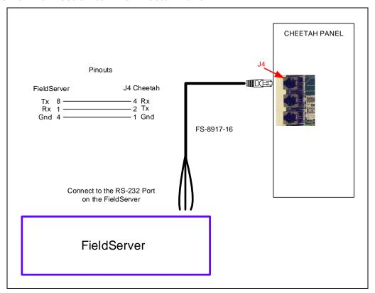
NOTE: RS-232 and RS-485 cannot be connected at the same time unless using the QS-2x10 QuickServer.
