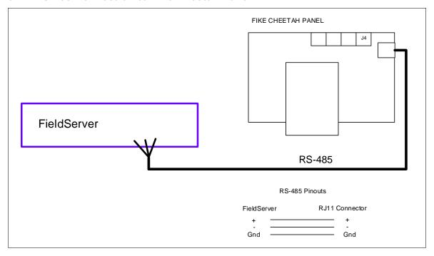
NOTE: RS-232 and RS-485 cannot be connected at the same time unless using the QS-2x10 QuickServer.
