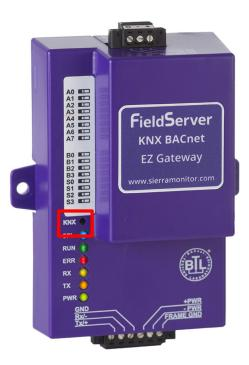
The KNX Administrator will request that the installer hit the service pin at the correct step of the commissioning process. Insert a small screwdriver or other device into the KNX port to activate the service pin when prompted.
