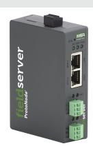
The QuickServer FS-QS-3X10-F series is available at four different point capacities. Each QuickServer is preloaded with 140 different drivers, such as Modbus, BACnet, SNMP, EtherNet/IP and many more. See page 3 for the complete list.
