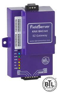
MSA Safety's unique FieldServer DeviceProxy™ feature allows each KNX device to be presented as a corresponding virtual BACnet device within the EZ Gateway, thereby providing granular visibility and control over each KNX device from within a BACnet management framework. For example, offline / online status is visible at the individual KNX device.
